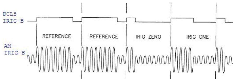
Specifically “IRIG-B” is defined by the code format IRIG-Bxyz, where x is the modulation type, y is the frequency and z is the coding. The two common types are:
