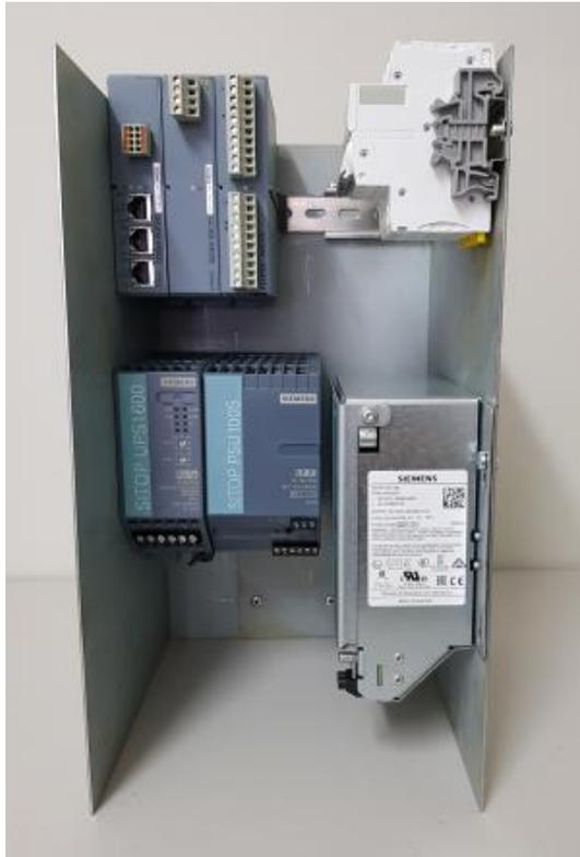
Figure 7. Automation controller, battery and charger – ready to fit in Transformer T panel.
