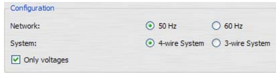
Figure 5. “Only voltages” PQ-Box 100 set-up
