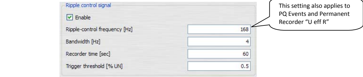
Figure 3. Ripple Control Signal setup dialog section of PQ-Box 100 Set-up “Basic settings”.
